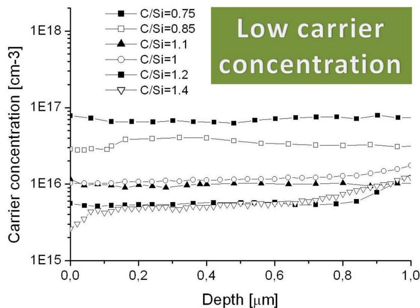
The quality of n-type epitaxial layers on on-axis 4H-SiC substrates is exceptionally high with EPD= 4·10<sup>3</sup>/cm<sup>2</sup>. Basal plane dislocations are completely eliminated. The surface morphology and screw dislocations density depend on substrate quality. Smooth areas (Ra=0.2nm) and island areas with SD in the center of an island (Ra=1.4nm), which are propagated from the substrate, can be observed on epilayers.
