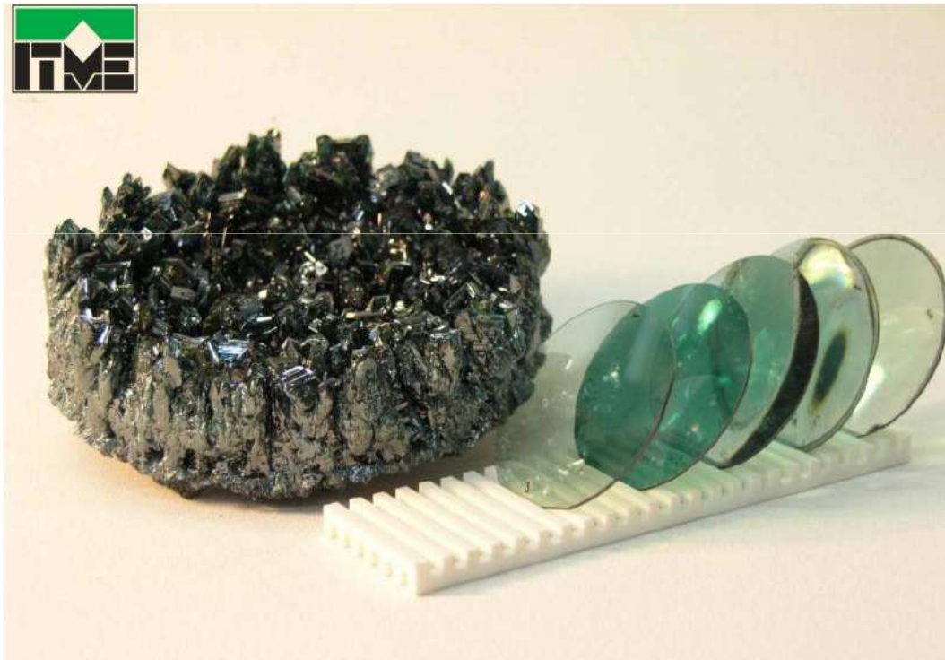
Silicon carbide polycrystal (left) and monocrystalline SiC wafers (right). Source: ITME
